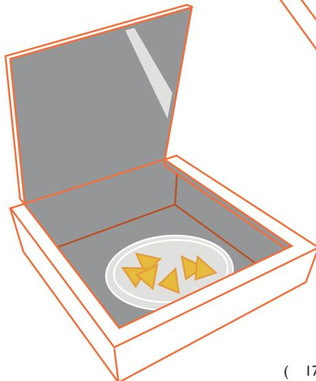
4) Tape plastic over the opening, which will help keep heat in, while allowing all the light to shine through. Then place a stick at an angle to prop the box up, helping reflect sunlight into the box.
