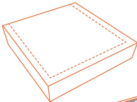
2) Cover the inside of the box and the flap with aluminum foil, gluing it down to make it as smooth as possible
