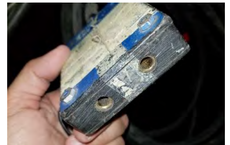
Bottom picture is the original two pin connector style without the third, ground pin. Top picture shows that the technicians tried to drill into the connector to allow the three pronged stage pin connector to be inserted
